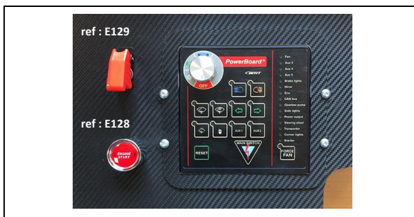
A03-2) Powerboard montée Powerboard mounted
